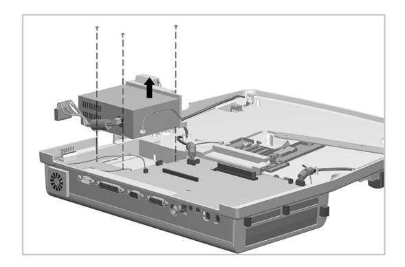
Figure 7-16. Removing the Power Supply Screws and Power Supply To install the power supply, reverse the procedure presented above. Be sure to reconnect the ground wire.
